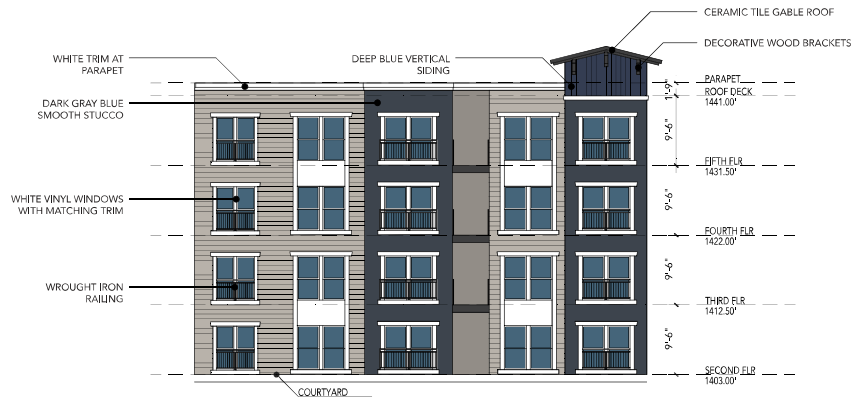
NORTH FACING ELEVATION
