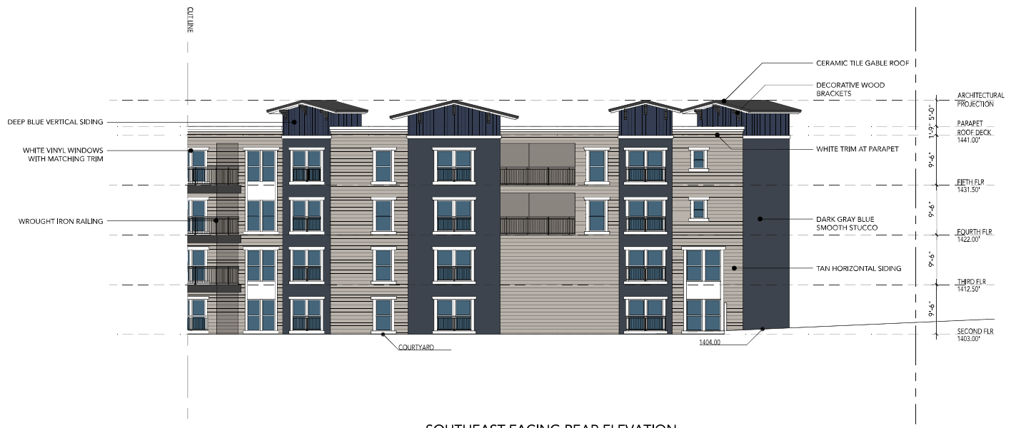
SOUTHEAST FACING REAR ELEVATION
