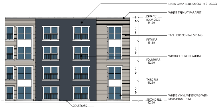
NORTH FACING ELEVATION
