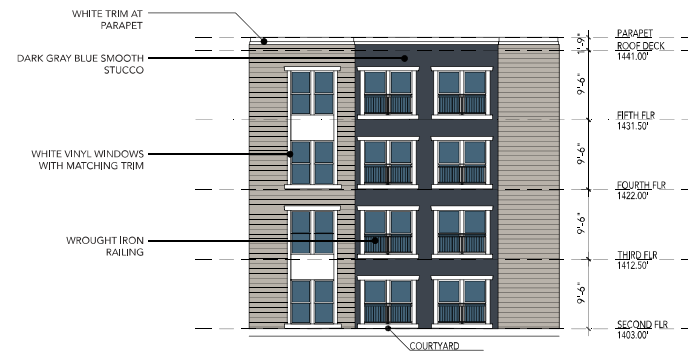
SOUTH FACING ELEVATION
